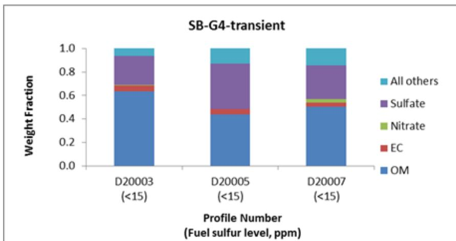
Figure 16. Intermediate Profiles Used for SB-G4-transient
