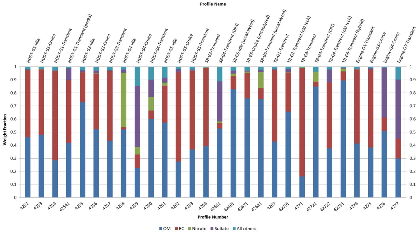
**Figure 2. Summary of the 28 composite V/E-MY/AT-Cycle speciation profiles (Based on a condensed set of the 5 species used in air quality modeling. Detailed species are maintained in the actual profiles.)**
