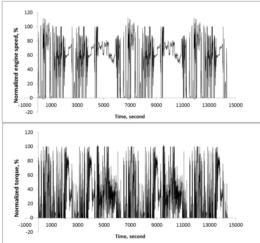
Figure A12. 4-hour Sub-cycle of 16-hour Cycle [10]
