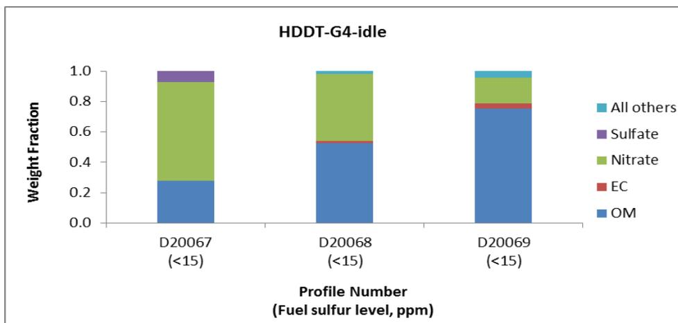
Figure 9. Intermediate Profiles Used for HDDT-G4-idle
