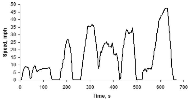
Figure A9. HHDDT Transient Cycle [19]
