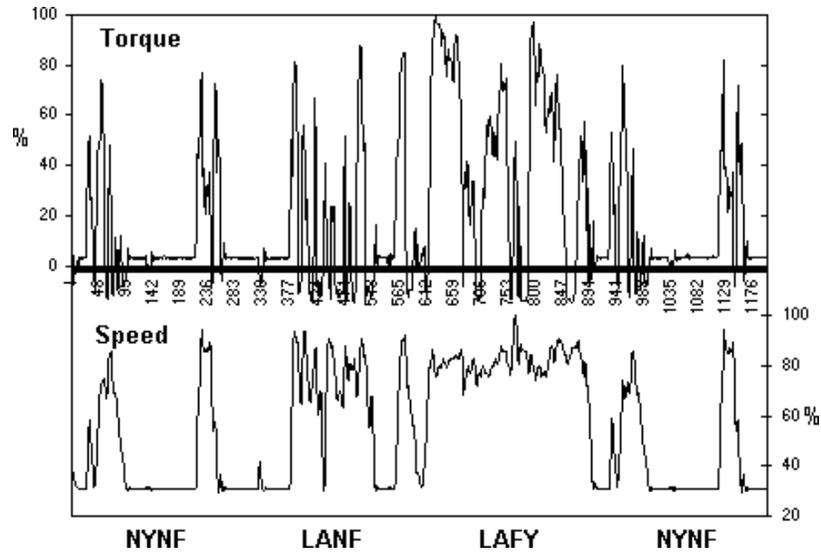
Figure A8. FTP Transient Cycle [19]
