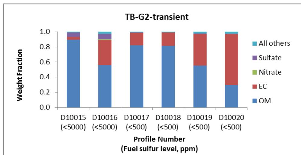
Figure 21. Intermediate Profiles Used for TB-G2-transient
